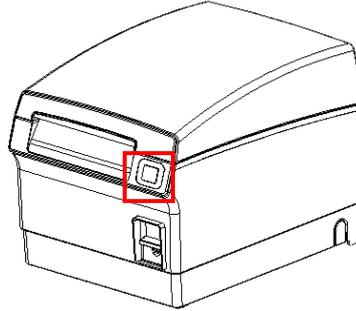
While the printer is turned off, turn on the printer while pressing the feed button. The printer setting values will then be printed with a beep sound.
