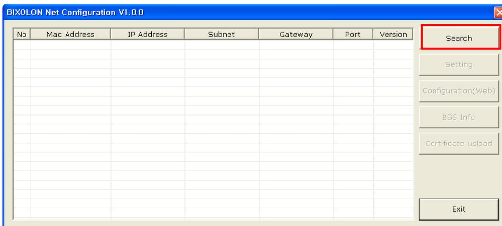
When you press the Search button, the SRP-F310 printer connected to the network will be shown in the list.
