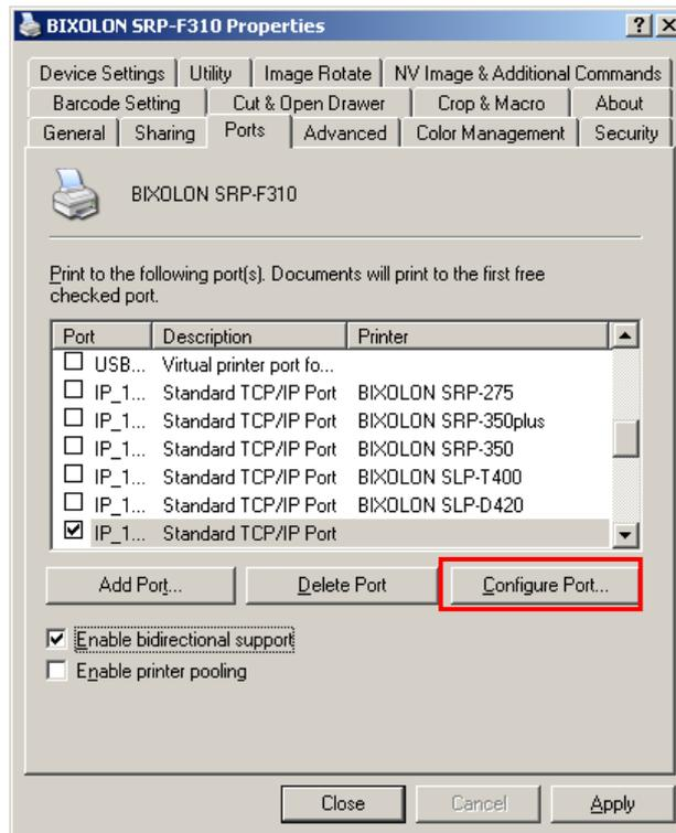
13) Enter the same number as the local port number set during the installation of the interface card in the “Port Number” field in the Raw Settings.
