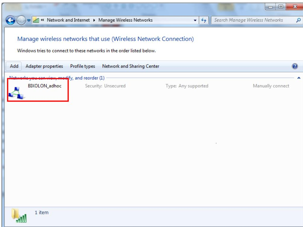
When the printer is set to the default value (Adhoc mode, SSID: BIXOLON\_adhoc), it will automatically connect.
