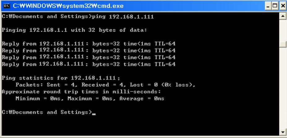
A screenshot of a Windows command prompt window titled "C:\WINDOWS\system32\cmd.exe". The prompt shows the command "ping 192.168.1.111" being executed. The output indicates a successful connection with four replies, each showing 32 bytes, a time of less than 1ms, and a TTL of 64. Ping statistics show 4 packets sent, 4 received, and 0% loss, with all round trip times being 0ms.
