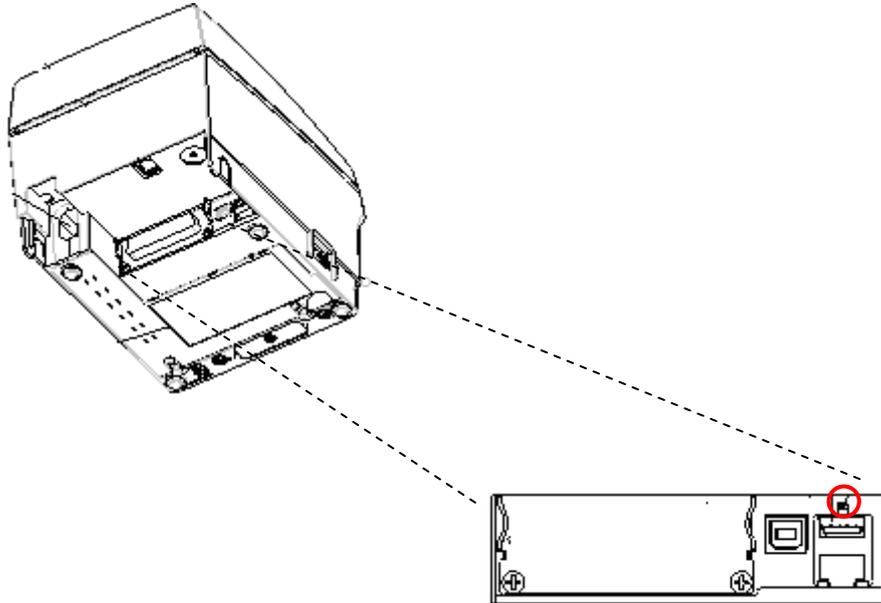
Pressing the Function Key while the power is ON will print the LAN/WLAN setting status page.
