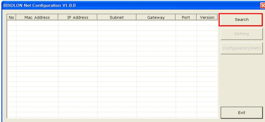
When you press the Search button, the SRP-F310 printer connected to the network will be shown in the list.
