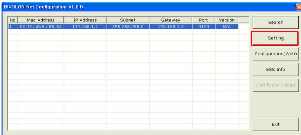
Select the SRP-F310 printer from the list and press the [Setting] button, and then the following window for changing the WLAN settings will pop up.
