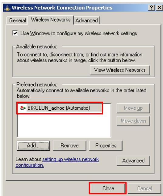
When the printer is set to the default value (Adhoc mode, SSID: BIXOLON\_adhoc), it will automatically connect.
