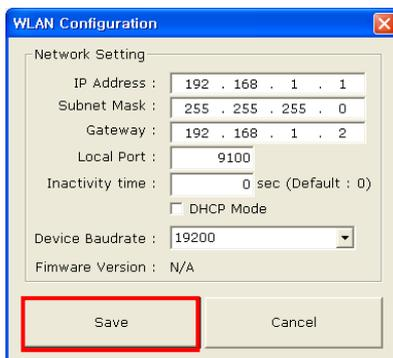
Enter the proper IP Address, Subnet Mask, and Gateway of the currently used network, and then click the [Save] button to save the settings.
