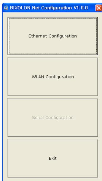
Click the Ethernet Configuration button when the printer is connected to the Ethernet, or click the WLAN button when the printer is connected through WLAN.
