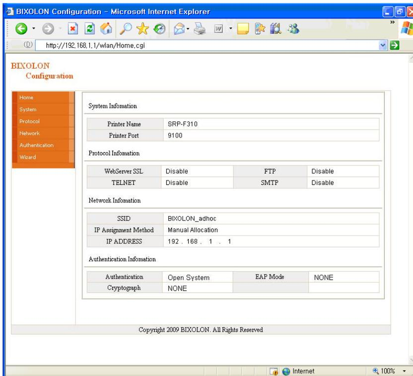
Home, System, Protocol, Network (WLAN), and Authentication can be configured from this window, and the wizard mode is also provided for easier step by step configuration.
